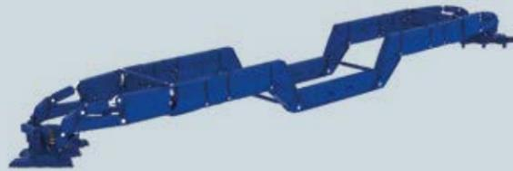
» With a payload of 350 t, the »FAKTOR« 5.5 high girder bridge can take on and transport up to 5,5 times its dead weight.
