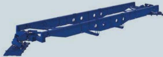
» The »FAKTOR« 5 high girder bridge, weighing just 100 t, combines low loading height and optimal load distribution with a maximum load capacity of impressive 500 t.
