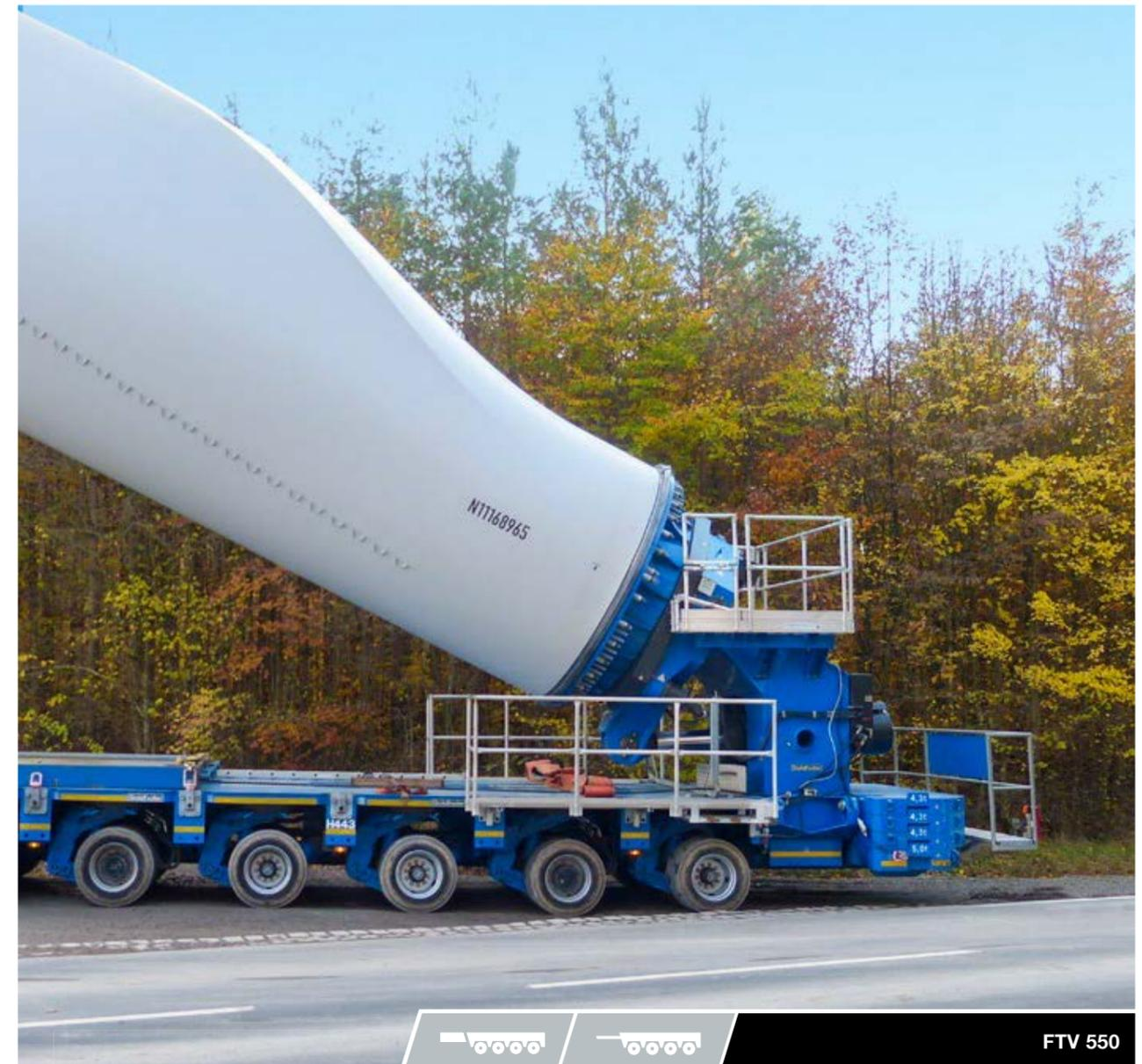
» Rotor blades of modern wind turbines can reach a length of 60 m or more. Rotor blade adapters with a diameter of up to 3.4 m are available to meet common blade type requirements.
